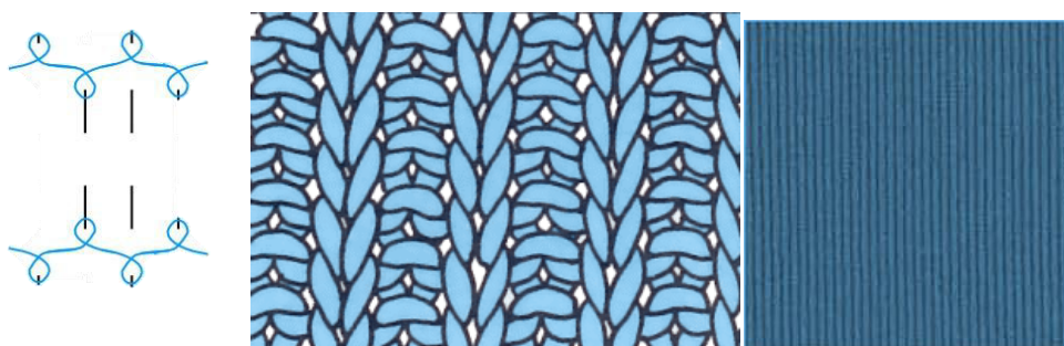
Figure. 2 Appearance of 1x1 ribbed knitwear and schematic formation of 1x1 ribbed knitwear
