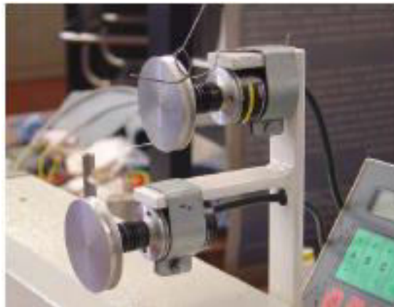
Figure 2: Encoder for measuring needle thread consumption on a lockstitch sewing machine
