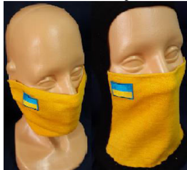
Figure. 1 - Production of textile samples of respiratory masks based on two-layer knitwear
