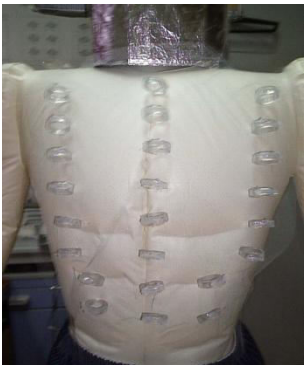
Figure. 2: Illustration of separation spacer placement on the chest of the thermal manikin
