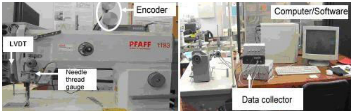
Figure 1: Positioning of the data collecting device on a lockstitch sewing machine
